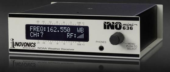
The INOmini 636 is a full-featured NOAA weather receiver in a small-format package. It tunes all weather band frequencies and delivers balanced analog and AES digital audio with automatic intelligibility enhancement for monitoring and rebroadcast. The 636 responds to the 1050Hz Alert Tone and provides alarm outputs for 1050Hz, plus audio and RF loss.
